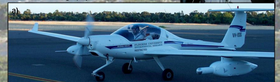
Fig 1: a) The Diamond ECO-Dimona Small Environmental Research Aircraft (SERA) platform, b) the cockpit with computer display of flight track and sensor output, and c) one of the two multipurpose instrument pods with the turbulence probe, attitude system and tri-spectral scanner installed.
